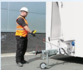
Unhitch from towing vehicle and operate hydraulics using the push button controls
